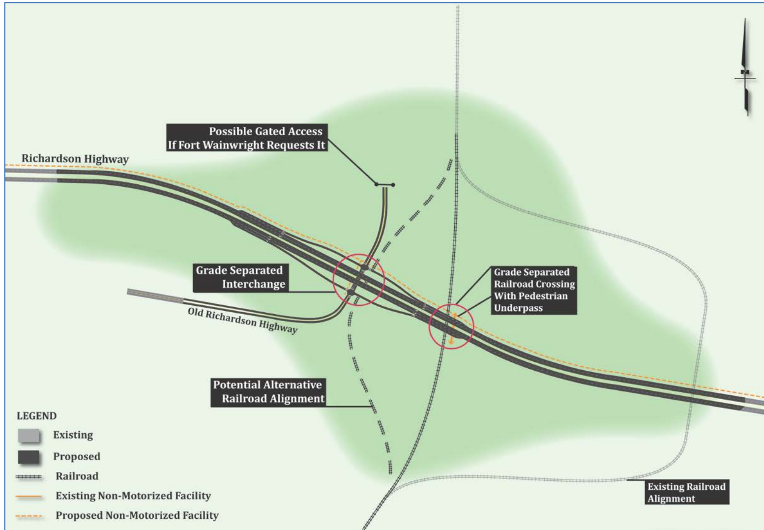
Figure 17 Concept 1 - Richardson Highway MP 359 Grade-Separated Facility
