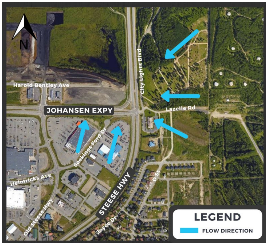
Figure 5. Existing Drainage patterns.
