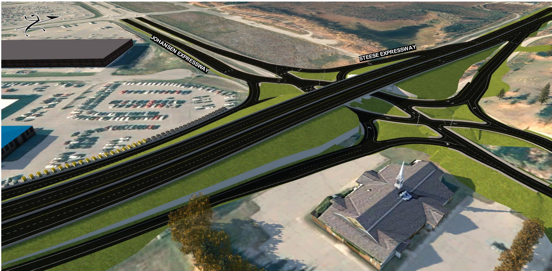
Figure 3.4: Diverging Diamond Interchange
