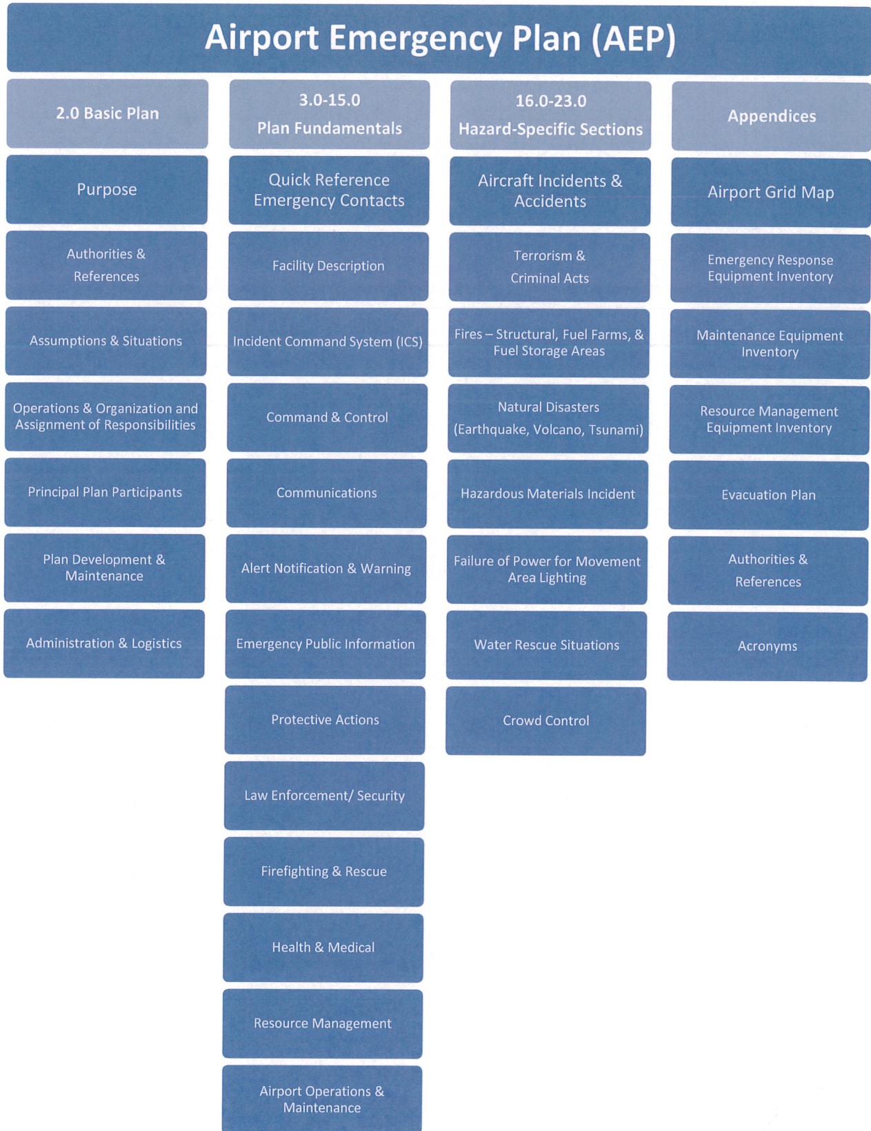
Figure 2-1: Airport Emergency Plan Structure
