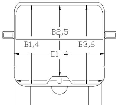
**OCCUPANT COMPARTMENT DEFORMATION MEASUREMENT**
