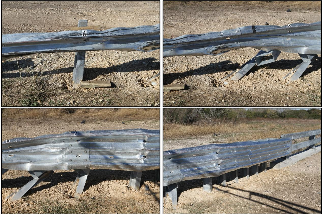
**Figure 7.5. Posts 6 through 15 after Test No. 608331-01-6.**
