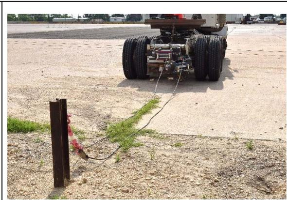
Typical Static Load Setup
