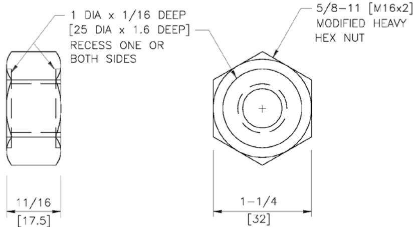
GUARDRAIL BOLT AND RECESSED NUT
