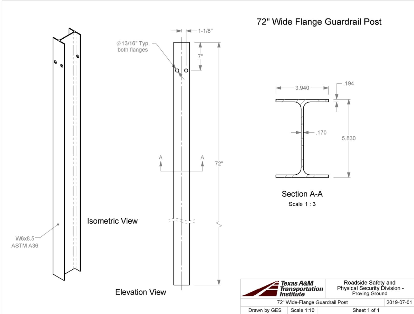
T:\Drafting Department\Solidworks\Standard Parts\Guardrail Parts and Subs\Guardrail Drawings\Post, 72" Wide Flange Guardrail
