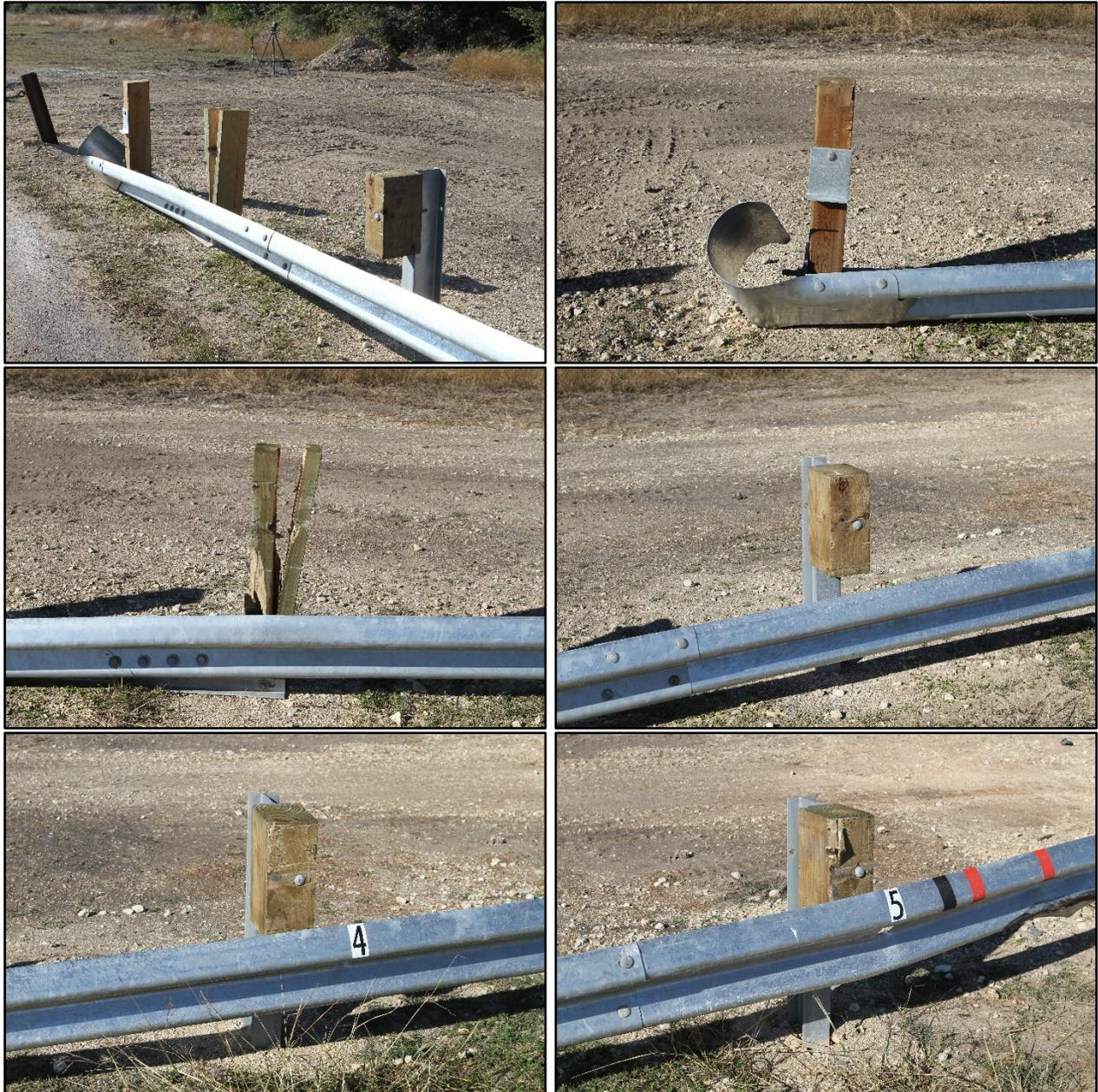
**Figure 7.4. Posts 1 through 5 after Test No. 608331-01-6.**
