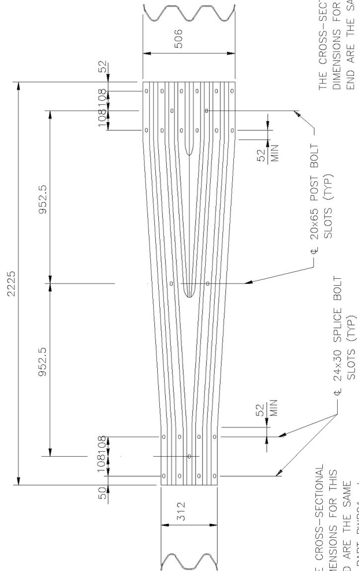
THE CROSS-SECTIONAL DIMENSIONS FOR THIS END ARE THE SAME AS PART RTM01a
