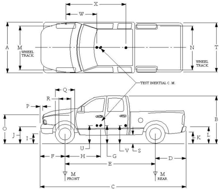
**Table F.2. Measurements of Vehicle Vertical CG for Test No. 608331-01-6.**
