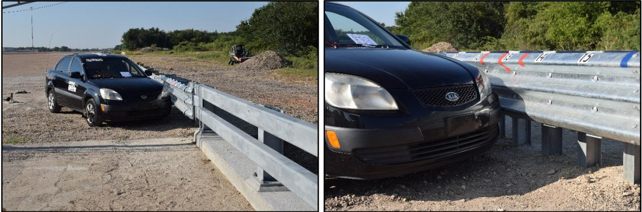
**Figure 5.1. Transition/Test Vehicle Geometrics for Test No. 608331-01-4.**
