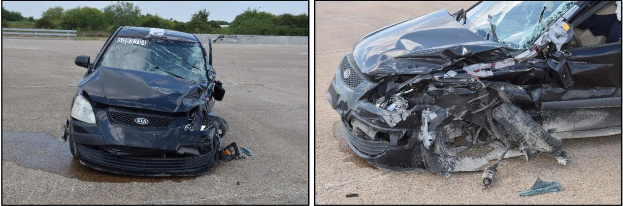
Figure 5.4. Test Vehicle after Test No. 608331-01-4.
