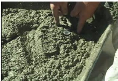
Pressing concrete around sensing device
