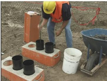
**Consolidation of concrete in cylinder by rodding**
