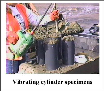
Vibrating cylinder specimens
